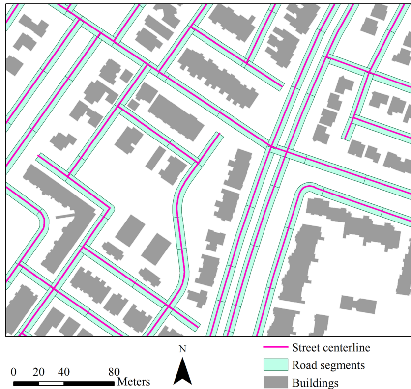
Figure 2. Map showing an example of road segments along the street centerlines for a small portion of the study area.
