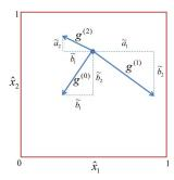
Figure 2. Safety box of a discrete time system consisting of two tasks.  $g^{(0)}$ ,  $q^{(1)}$  and  $q^{(2)}$  are the possible movements.
