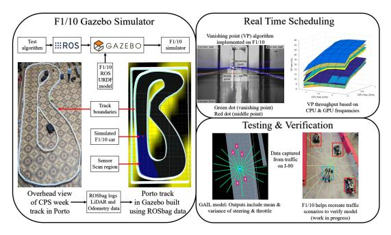
Figure 5: Figure (left) shows an F1/10 car in a simulated environment generated using data from the real world, (right, top) real time scheduling of vanishing point algorithm on the F1/10 onboard computer and, (right, bottom) verifying traffic behavior
