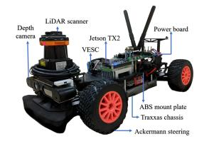
Figure 1: It takes only a couple of hours fully to assemble a F1/10 autonomous racecar, using detailed instructions available at http://f1tenth.org/
