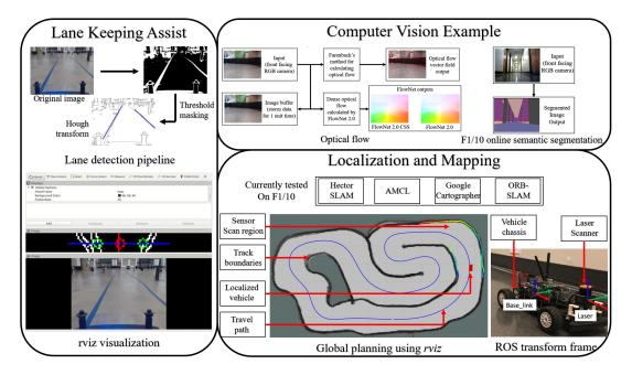
Figure 4: Some perception research enabled by the F1/10 platform (clockwise, starting left); (a) lane following using a monocular camera, (b) optical flow computation using Farenback's method and FlowNet 2.0 and, (c) localization and mapping
