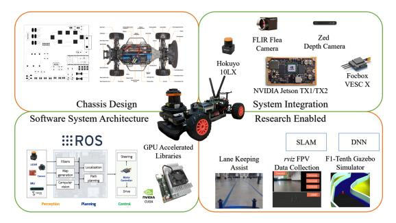
Figure 2: Overview of the F1/10 research instrument - Modular chassis and system design with detailed instructions; open-source software stack in ROS; and a wide variety of AV research enabled in the lab on a real testbed.
