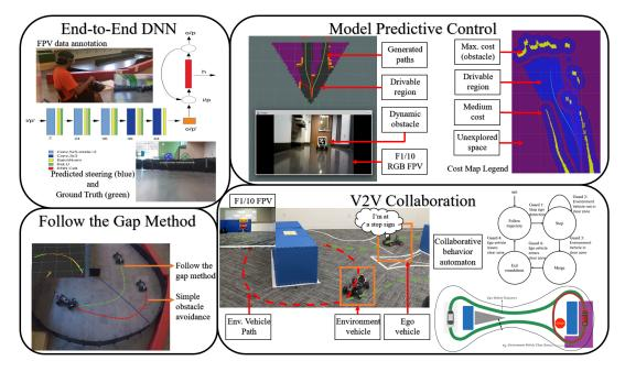
Figure 3: Planing and control research enabled by the F1/10 platform: (Bottom Left) Reactive Obstacle Avoidance, (Top Left) End-to-End Driving, (Top Right) Model Predictive Control, (Bottom Right) V2V Collaboration
