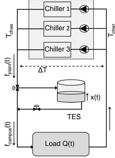
Fig. 3. Model of a single plant containing 3 chillers and a TES system. Chilled water  $T_{chws}$  flows from the chiller towards the load. Charging and discharging of the TES takes place through control valves and changes the height  $x(t)$  of the water column inside the TES.
