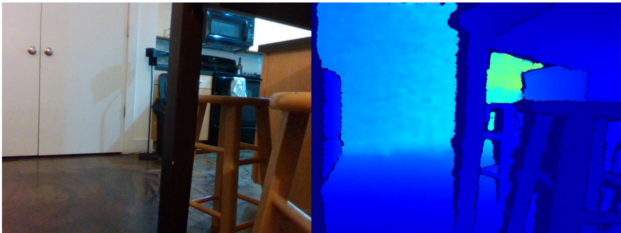
Images provided by the RealSense D435 camera showing both an RGB image (left) and the depth view of the same scene generated by its depth cameras (right).
